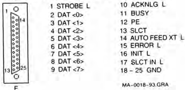
Figure B-3 Parallel Printer Port (Bidirectional)
